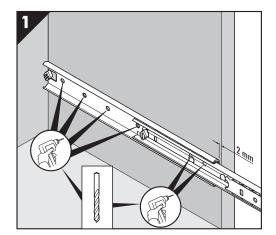
Marking holes to fix the external member of the slide to the cabinet.
